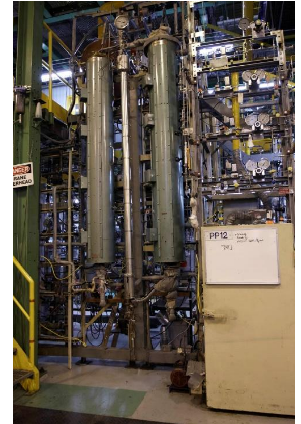
Pilot-scale unit for co-processing and SAF technology development
