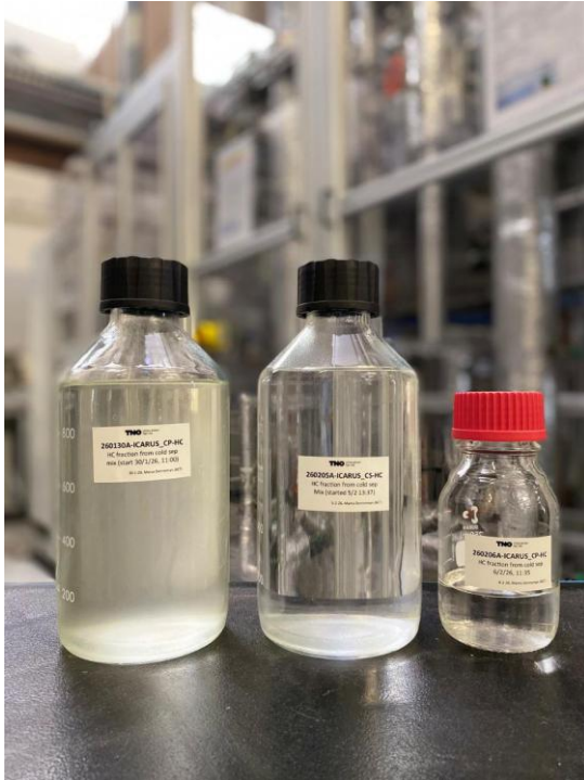
2 L of liquid produced (Olefin-rich SAF precursor)
